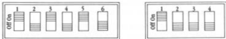
Figure 3-12. Switch Settings for Epson Printers
